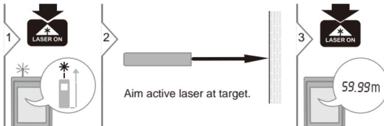
**i** Target surfaces: Measuring errors can occur when measuring to colourless liquids, glass, styrofoam or semi-permeable surfaces or when aiming at high gloss surfaces. Against dark surfaces the measuring time increases.
