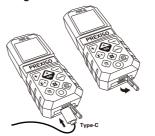
Open the cap and insert the USB recharging cable with Type-C Port
