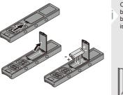
Change batteries when battery symbol is empty.
